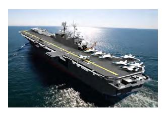
The new big-deck assault ship Tripoli will not feature a well deck, allowing more space for aircraft and aviation facilities.
